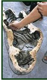
2. Liquid wax is painted on then poured into the rubber mold, coating the mold’s surface.
