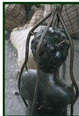
5. The wax impression is then encased, layer upon layer, with a special mix of refined plaster and other materials, which hardens into an “investment casting” mold.
